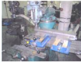
Surface milling on #8
