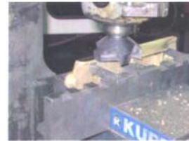
Surface milling on #4
